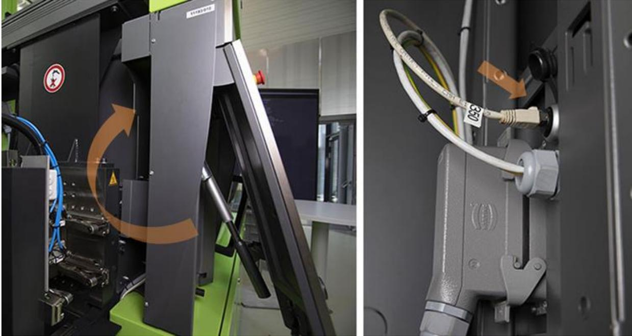
Please make sure that the machine is connected to your local network with a proper Ethernet cable through the *eth0* network interface (RJ45 connector) on the backside of the control panel.
